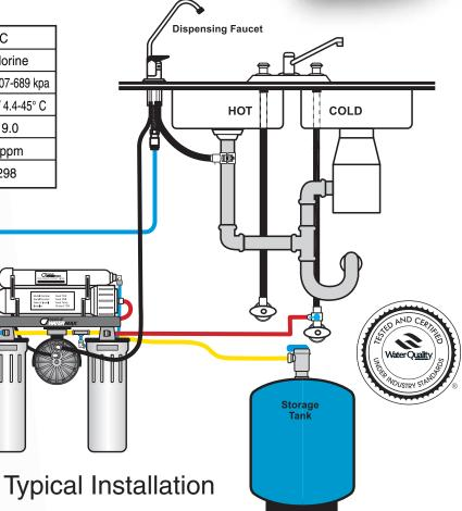
Do not use with water that is micro biologically unsafe or of unknown quality without adequate disinfection before and/or after the system. Do not freeze or plumb to hot water.
